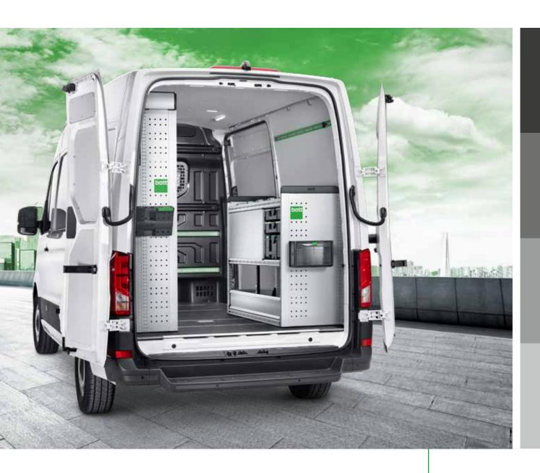
The bott vario3 van racking modules for your commercial vehicle offer versatile components for dividing the storage space. These can be easily adapted to the individual requirements of your trade. The bott vario3 van racking designers paid particular attention to safety, functionality and to making optimum use of the available space.
