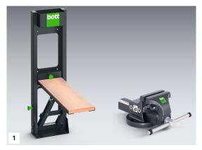
1 Set comprising: Folding worktop incl. vice - for working outside the vehicle Zinc-plated sheet steel, beech multiplex worktop Jaw width 125 mm, weight 24 kg
